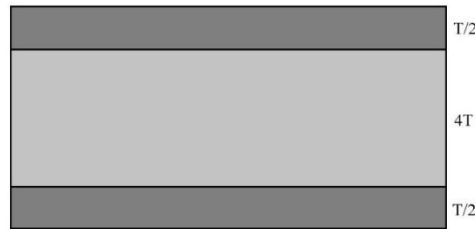
Figure (19): Honeycomb Sandwich Skin Core Thickness Ratio [42]
