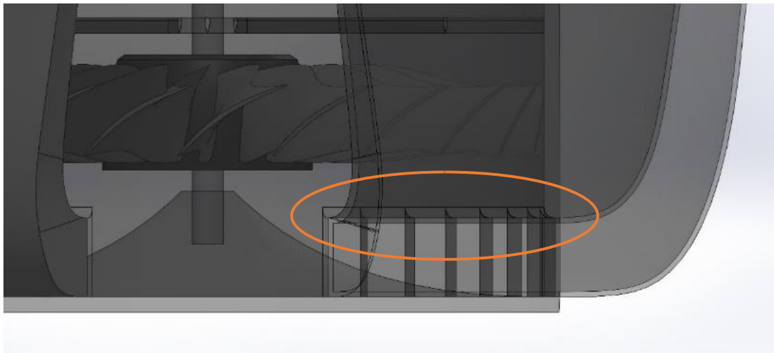
Figure (24): Outlet Air Duct Opening
